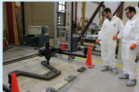
Dana C. Wood Materials and Structures Laboratory—3D Concrete Printer
